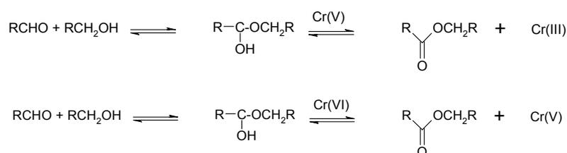
**Scheme 2.** Aldehyde oxidation mechanisms (R = tridecyl).
