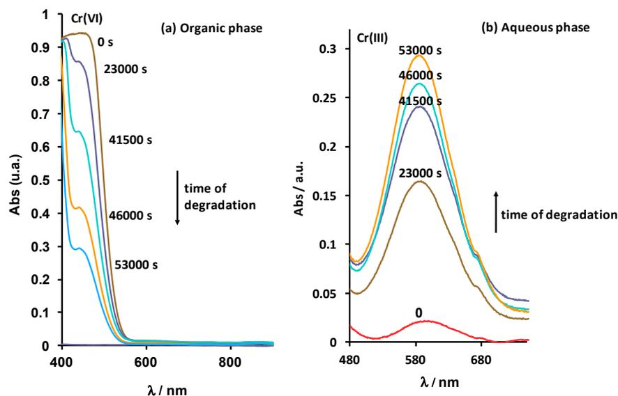
**Figure 2.** (a) UV-Visible spectra of the organic phase throughout the degradation (organic phase contained initially  $0.2 \text{ mol}\cdot\text{kg}^{-1}$  tri-*n*-octylamine diluted in *n*-dodecane modified with 5 wt % 1-tridecanol +  $0.05 \text{ mol}\cdot\text{kg}^{-1}$  Cr(VI); (b) UV-Visible spectra of the aqueous phase in contact with the organic phase throughout the chemical degradation of the organic phase. Temperature =  $25 \text{ }^{\circ}\text{C}$ .
