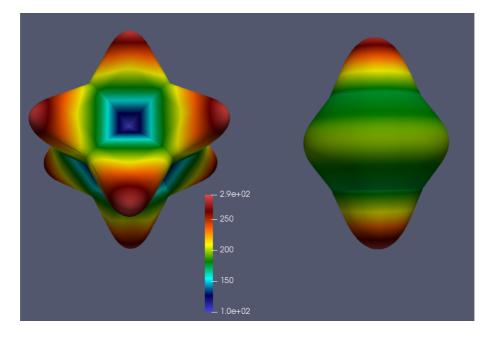
Figure 3: On the left, magnitude of the directional Young modulus of the FCC phase of an austenitic steel in all the space directions considering  $c_{11}^* = 197.5$  GPa,  $c_{12}^* = 125$  GPa and  $c_{44}^* = 122$  GPa [Sau06]. On the right, magnitude of the directional Young modulus of the corresponding HCP phase computed from Eq.9. The vertical axis is aligned with the  $\langle 111 \rangle_{\gamma}$  and  $\langle 0001 \rangle_{\varepsilon}$  crystallographic directions, respectively.
