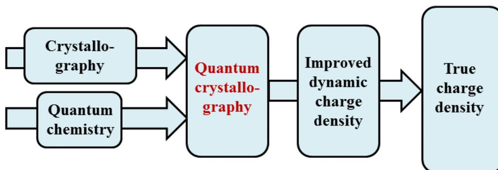
**Figure 2.** Quantum crystallography, second aspect: quantum chemical calculations are integrated into crystal structure determination to improve the dynamic charge density, i.e. the thermally smeared electron and nuclear densities.
