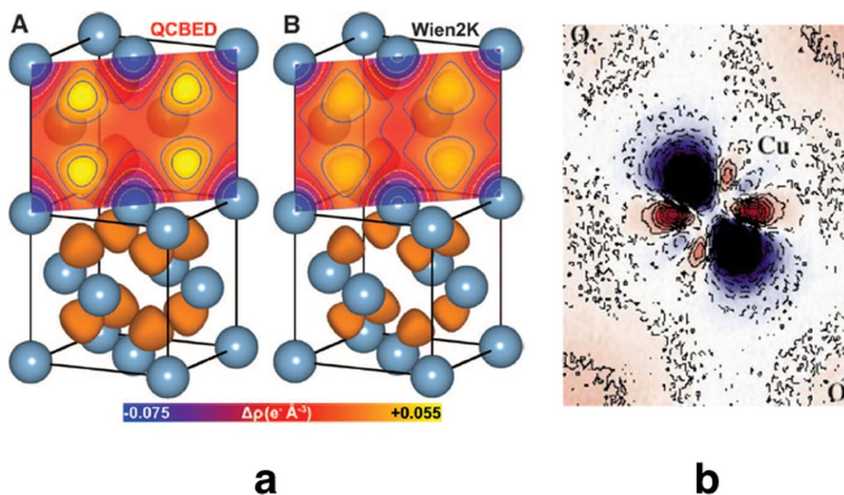
**Figure 8:** a) Electron density of aluminium from quantitative CBED (left) and a periodic plane-wave calculation using the program Wien2k (right). Reprinted from ref. 120 with permission from AAAS. b) Static deformation density map around a copper atom in  $\text{Cu}_2\text{O}$ . Reprinted by permission from Macmillan Publishers Ltd.: *Nature*, ref. 122, copyright 1999.
