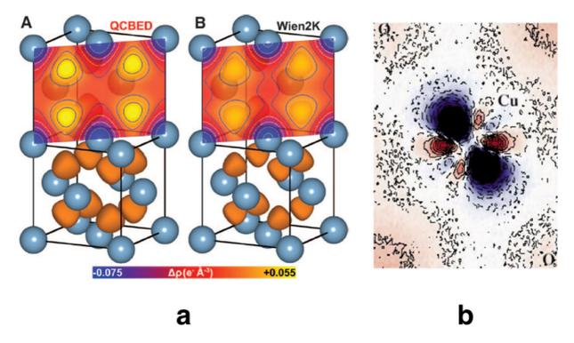
**Figure 8**: a) Electron density of aluminium from quantitative CBED (left) and a periodic plane-wave calculation using the program Wien2k (right). Reprinted from ref. 120 with permission from AAAS. b) Static deformation density map around a copper atom in Cu<sub>2</sub>O. Reprinted by permission from Macmillan Publishers Ltd.: *Nature*, ref. 122, copyright 1999.
