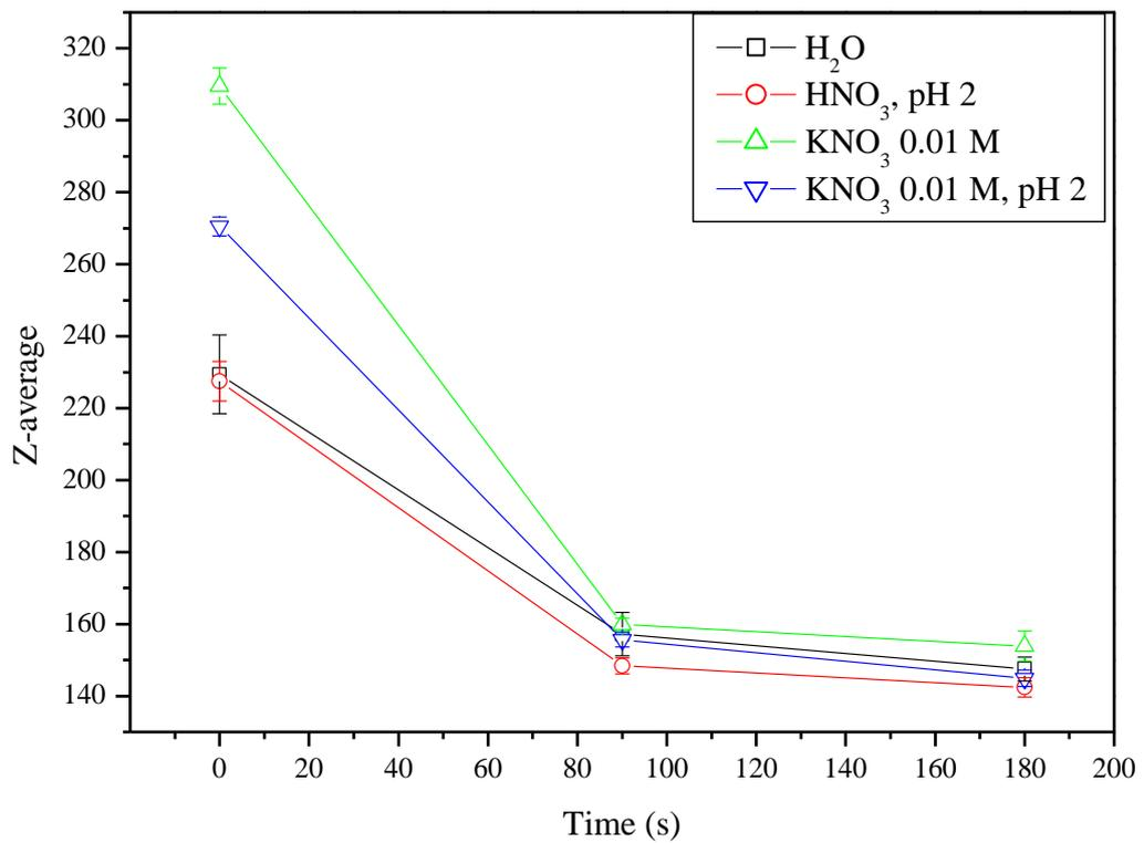
Figure 6 : Evolution of mean alumina nanoparticle size in different suspensions versus ultrasonic time.
