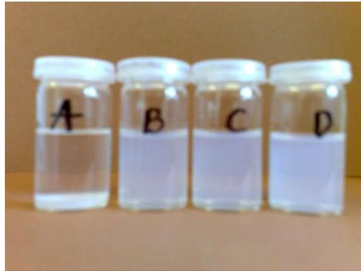
Figure 7: Alumina suspensions after ultrasonication 30 min (A) pH 2, H<sub>2</sub>SO<sub>4</sub>; (B) pH 2, HNO<sub>3</sub>; (C) KNO<sub>3</sub> 0.01 M; (D) pH 2, HNO<sub>3</sub> and KNO<sub>3</sub> 0.01 M.
