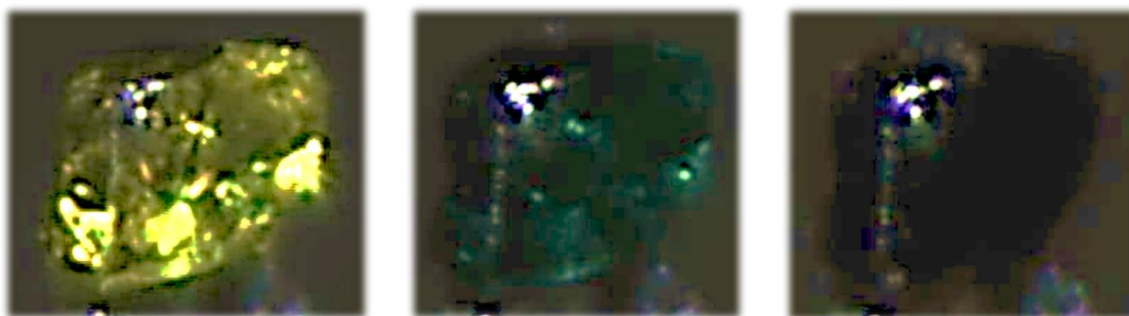
Figure S3. The color of single crystal of [\text{RuNOPy}_4\text{F}](\text{ClO}_4)_2 complex in GS (left, yellow), MS1 (middle, deep green) and MS2 (right, black).
