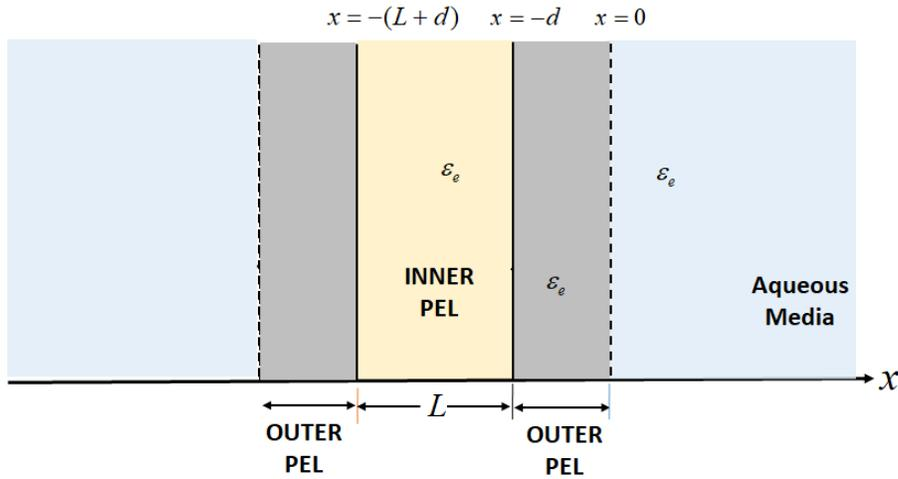
**Fig. 1.** Schematic illustration of a core-shell particle consisting of an inner polyelectrolyte layer (PEL in short) of thickness  $L$  (core component) covered by a peripheral PEL (shell component) of thickness  $d$ . Details on the adopted nomenclature are provided.
