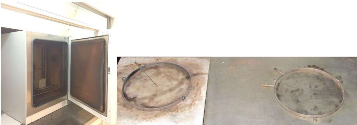
Figure 2: Insulated oven of 125L (left), ceramic insulating plate (middle) and metal plate (right)
