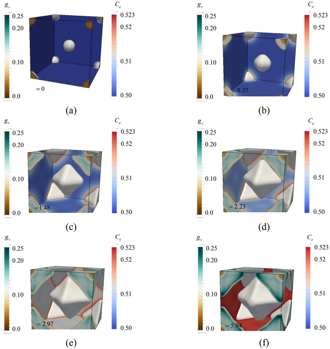
Figure 4. Mesoscopic simulation results showing solid fraction  $g_s$  (plotted in the interior of the envelopes) and solute concentration in the extra-dendritic liquid  $C_e$  (plotted in the exterior of the envelopes) at different non-dimensional times  $\tau = tV_h^2(\tau_0)/D_l$ : (a)  $\tau = 0$ , (b) 0.37, (c) 1.48, (d) 2.23, (e) 2.97, and (f) 5.94. This simulations is for the isothermal case with low undercooling ( $\tau_0 = 0.05$ ) and high grain density ( $R_f/D_l/V_h(\tau_0) = 4.03$ ).
