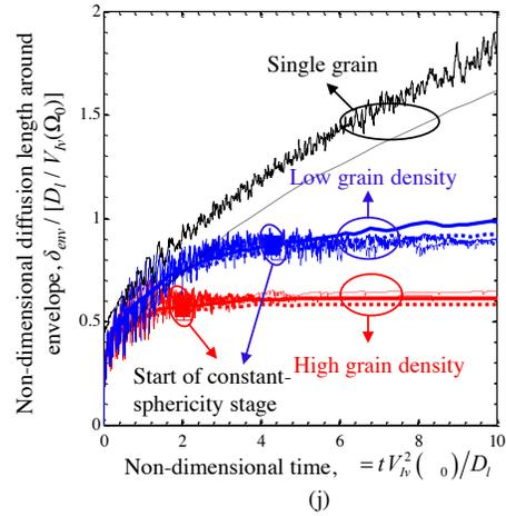
Figure 6. (a-j) Upscaled mesoscopic results plotted as a function of non-dimensional time. High and low grain density cases correspond to  $R_f / D_l / V_{lv}(\omega_0) = 4.03$  and  $6.31$ , respectively.
