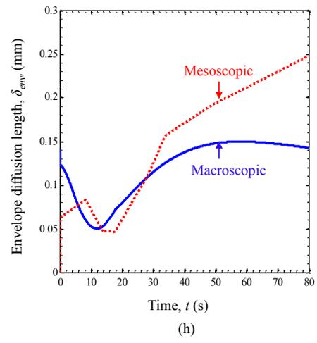
Figure 15. Comparison between the mesoscopic and macroscopic quantities plotted as a function of time. This comparison is for the recalescence case with intermediate grain density:  $R_f = 1.6 \text{ mm}$ .
