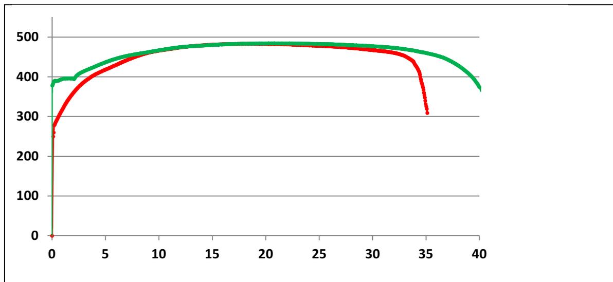
**Figure 3:** Engineering stress (MPa),  $\sigma_{eng}$ , versus engineering strain in %,  $\varepsilon_{eng}$ , for the two specimens R\_21.3 (red curve) and R\_2.8 (green curve).
