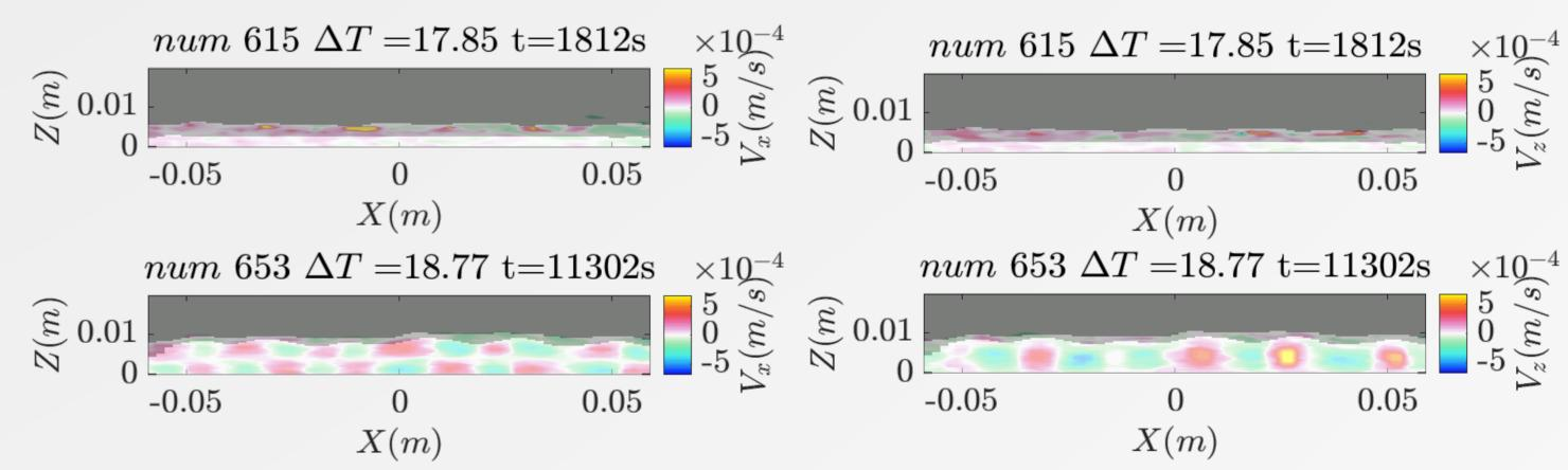
Maps of the horizontal (left) and vertical (right) velocities in the fluid with two temperature differences
