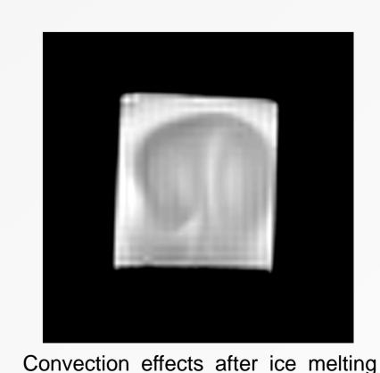
in supercooled water experiments.
