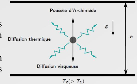
$Ra = \frac{\rho g \beta \Delta T h^3}{\mu \kappa}$  with  $\rho$  the density of the liquid, g the gravity,  $\beta$  the thermal expansion coefficient,  $\mu$  the fluid viscosity and  $\kappa$  the thermal diffusivity
