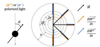
FIG. 3. Sketch of the induced magnetization produced by  $\sigma^+$  and  $\sigma^-$  polarized light per unit of time for different orientations of the magnetic moments with respect to the direction of propagation of the light. The parameters  $\alpha$ ,  $\beta$ , and  $\gamma$  of the fitting law defined by Eq. (6) are represented.
