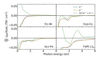
FIG. 1. Continuous lines: Variation of the magnetization with respect to time induced by optical transitions in fcc Ni, hcp Co, bcc Fe, and FePt  $L1_0$  for circularly left and right polarized light,  $\sigma^+$  and  $\sigma^-$ . Dashed line: Difference of the variation of the magnetization induced by  $\sigma^+$  and  $\sigma^-$  polarized light with respect to time scaled by a factor 10.
