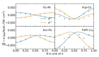
FIG. 4. Markers: Angle-dependent part of the magnetization induced by  $\sigma^+$  and  $\sigma^-$  polarized photons of 1.55 eV per unit of time for different values of  $\theta$ , the angle between the light propagation axis and the magnetization. Continuous lines: Fit using Eq. (6) and the values of  $\alpha$ ,  $\beta$ , and  $\gamma$  given in Table I.
