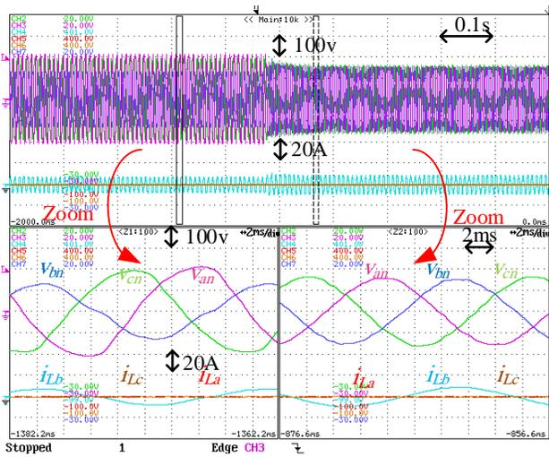
Fig. 13. Experimental results: load voltages and currents during steady state with unbalanced resistive loads ( $R_a = R_b = \infty \Omega$  and  $R_c = 15 \Omega$ ) before and after activating the proposed control.
