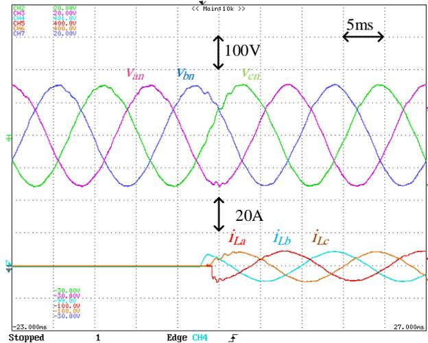
Fig.14. Transient of 0%–100% balanced resistive load.
