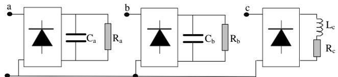
Fig. 16. Topology of the tested unbalanced nonlinear loads.
