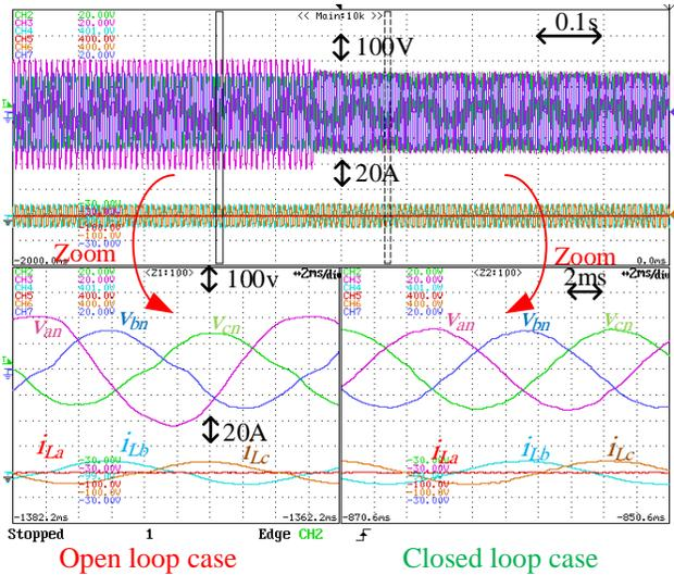
Fig. 12. Experimental results: load voltages and currents during steady state with unbalanced resistive loads ( $R_a = \infty \Omega$  and  $R_b = R_c = 15 \Omega$ ) before and after activating the proposed control.
