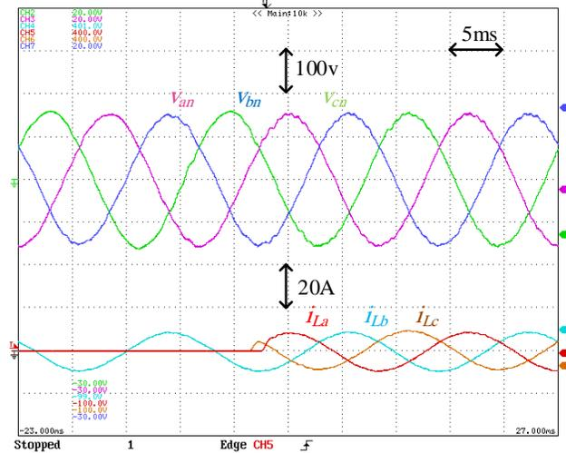
Fig. 15. Transient of single phase load to balanced resistive load.
