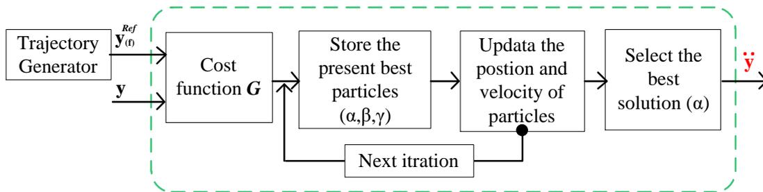
Fig. 4. Block diagram of the GW based tracking controller.
