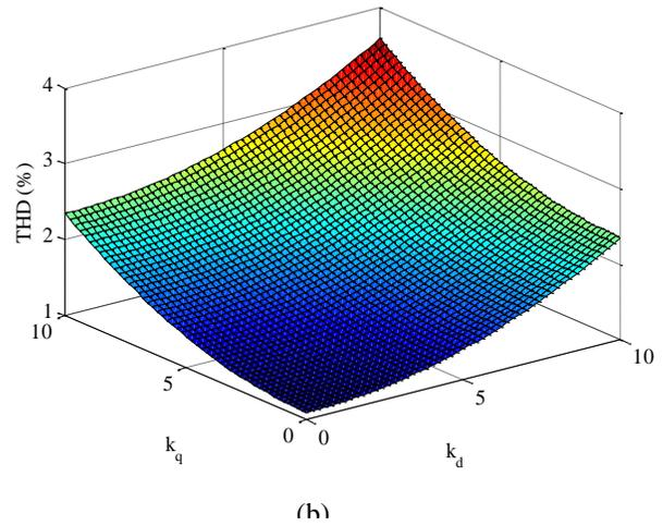
Fig. 5. Influence of the cost function odq-axis parameters on the voltage THD evolution: (a)  $k_0$  gain influence when gains  $k_d$  and  $k_q$  are set equal, (b)  $k_d$  and  $k_q$  gains influence when  $k_0$  is set to 10.
