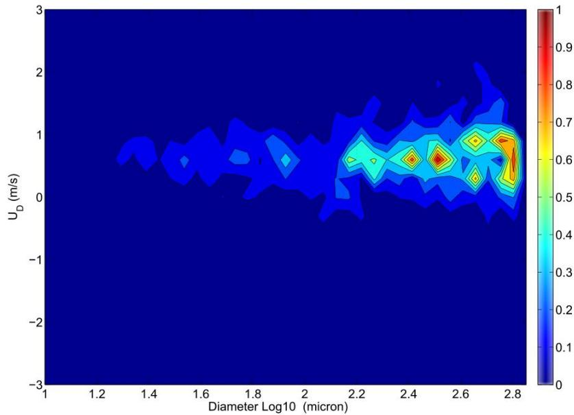
**Figure 5.** Size-Velocity measurements obtained from the PDA analysis. Measurement point is located 10 cm below the injector, 1 cm slightly off axis.
