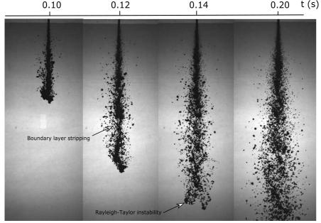
Figure 3. Shadowgraph images for D2P6 experiment.
