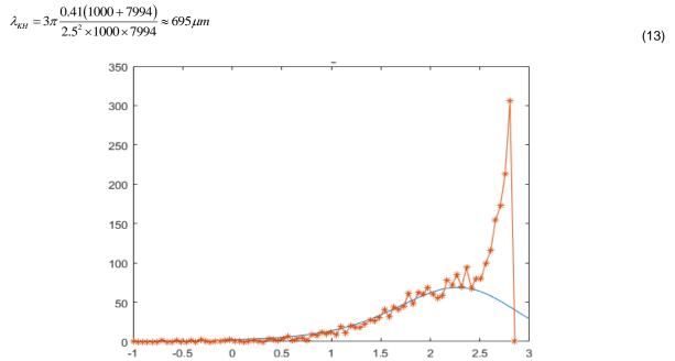
Figure 6. Number of droplets collected by the PDA according to the logarithm of their size.
