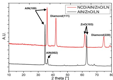
**Figure 10** XRD diffraction patterns of S3 sample (AlN-coated ZnO/LiNbO<sub>3</sub>) before and after NCD growth.
