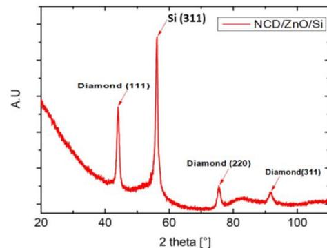
**Figure 4** XRD pattern of S1 sample (ZnO/Si) after NCD growth.
