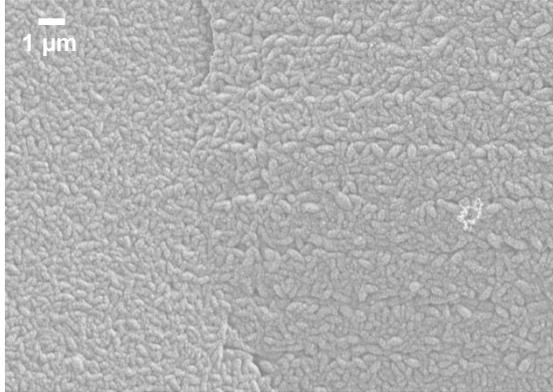
**Figure 12** SEM micrograph (secondary electrons) of the IDTs base (on the left) and the IDTs fingers (on the right) of the NCD/AlN/ZnO/IDTs/LiNbO<sub>3</sub> WLAW device achieved on S4 sample.
