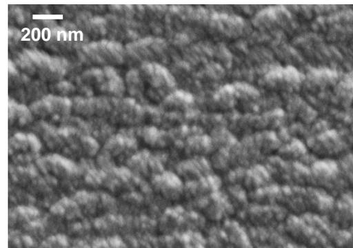
**Figure 8** SEM micrograph of NCD film deposited on S3 sample (AIN-coated ZnO/LiNbO<sub>3</sub>).
