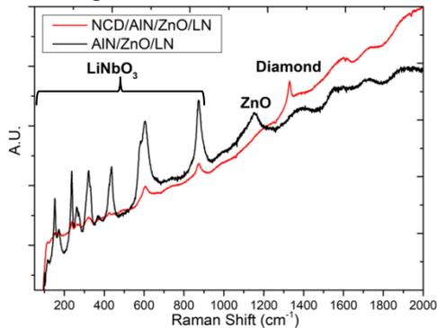
**Figure 9** Raman spectra of S3 sample (AlN-coated ZnO/LiNbO<sub>3</sub>) before and after NCD growth.
