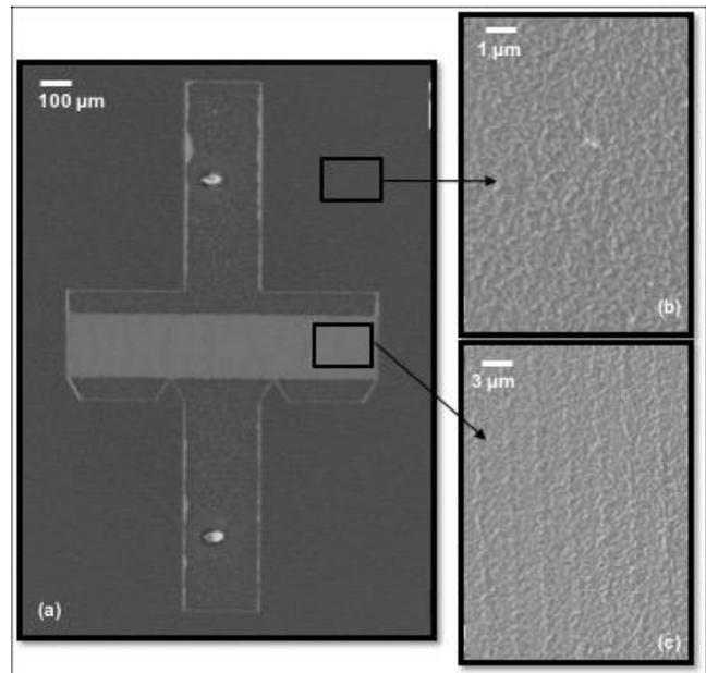
**Figure 11** SEM micrograph (back-scattered electrons) of the NCD/AlN/ZnO/IDTs/LiNbO<sub>3</sub> WLAW device achieved on S4 sample: (a) global view; (b) focus out of the device; (c) focus of the IDTs finger zone.
