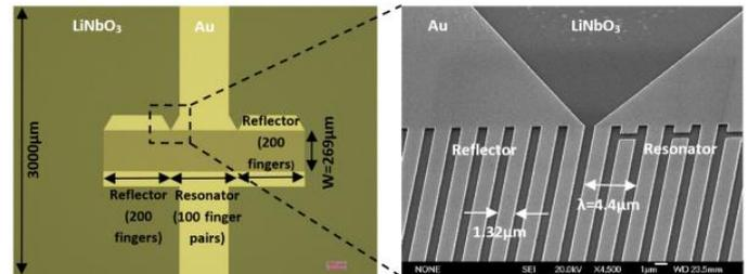
**Figure 1** Top view of a microfabricated SAW device formed of IDTs(Ti/Au)/LiNbO<sub>3</sub> before ZnO deposition.
