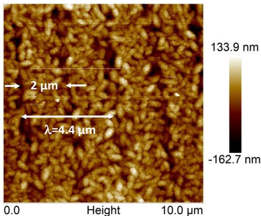
**Figure 13** AFM micrograph of the IDTs finger zone of the NCD/AlN/ZnO/IDTs/LiNbO<sub>3</sub> WLAW device realized on S4 sample.
