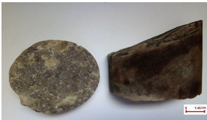
Fig. 2. Photograph of core samples used for laboratory measurements before preparation.
