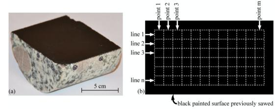
$\label{eq:scalar} Fig. 3. (a) Photograph of a granites ample prepared for measurement, (b) Schematic representation of the sample's scanned surface, indicating the position of the multiple of the sample of the$
