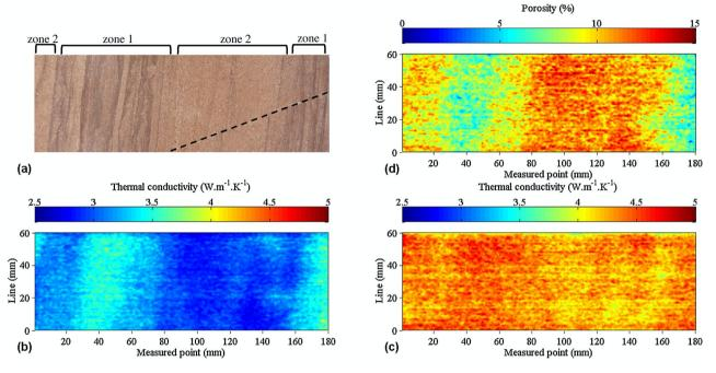
Fig. 2. (a) Analyzed surface of the sandstone sample; black dotted line indicates the sealed fault; (b) Measured thermal conductivity map of the air saturated sandstone sample; (c) Measured thermal conductivity map of the water saturated sandstone sample; (d) Computed porosity map of the sandstone sample.
