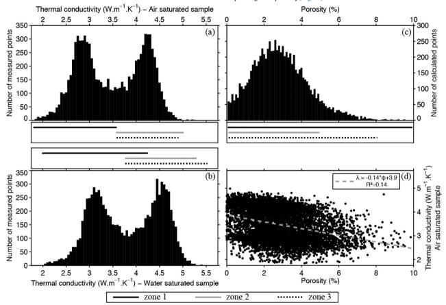
Fig. 4. Granite sample: (a), (b), distribution of measured thermal conductivity values, in the air and water saturated sample respectively (column width: 0.05Wm-1K-1);
