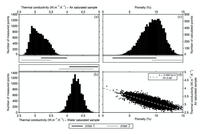
Fig. 5. Sandstone sample: (a), (b), distribution of measured thermal conductivity values, in the air and water saturated sample respectively (column width: 0.05Wm-1 K-1);
