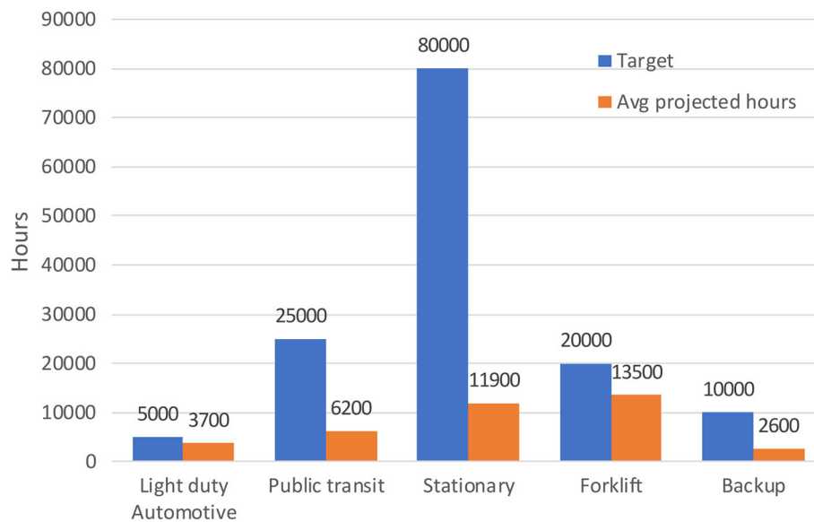
Fig. 5 Lab data projected hours to 10% stack voltage degradation [26]
