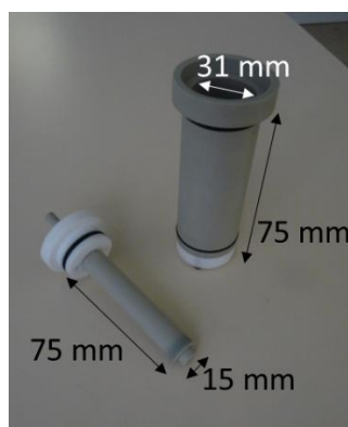
Figure 1. Polypropylene Couette geometry used to perform the experiments in the MRI and in the conventional rheometer.
