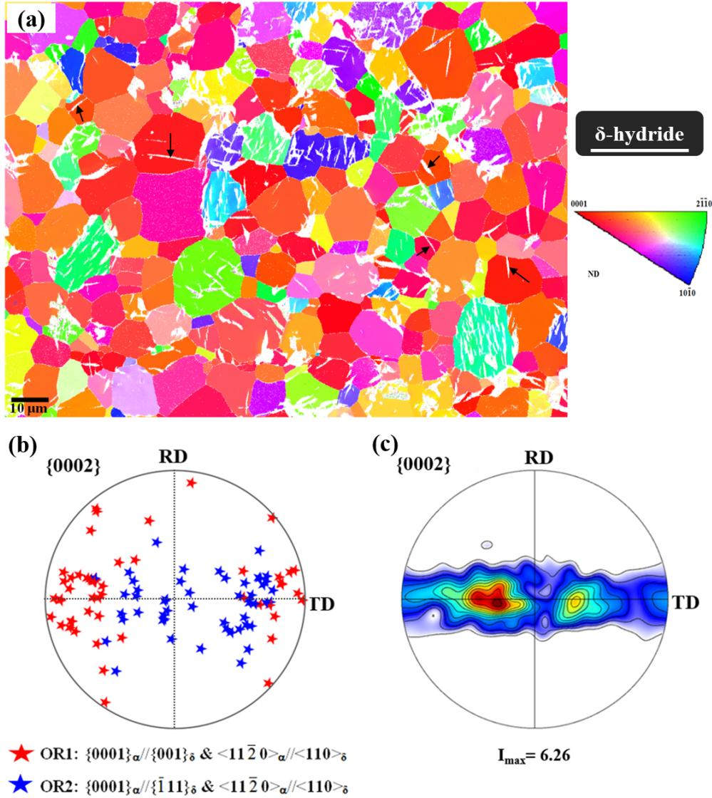
Fig. 6 Correlation between hydride precipitation and grain orientation. (a) IPF map of the matrix of the Ti50A-H, the  $\delta$ -hydride ( $TiH_{2-x}$ ) indicated by white color; (b)  $\{0002\}$  pole figure of grains following OR1 and OR2; (c)  $\{0002\}$  pole figure of AR-Ti50A.
