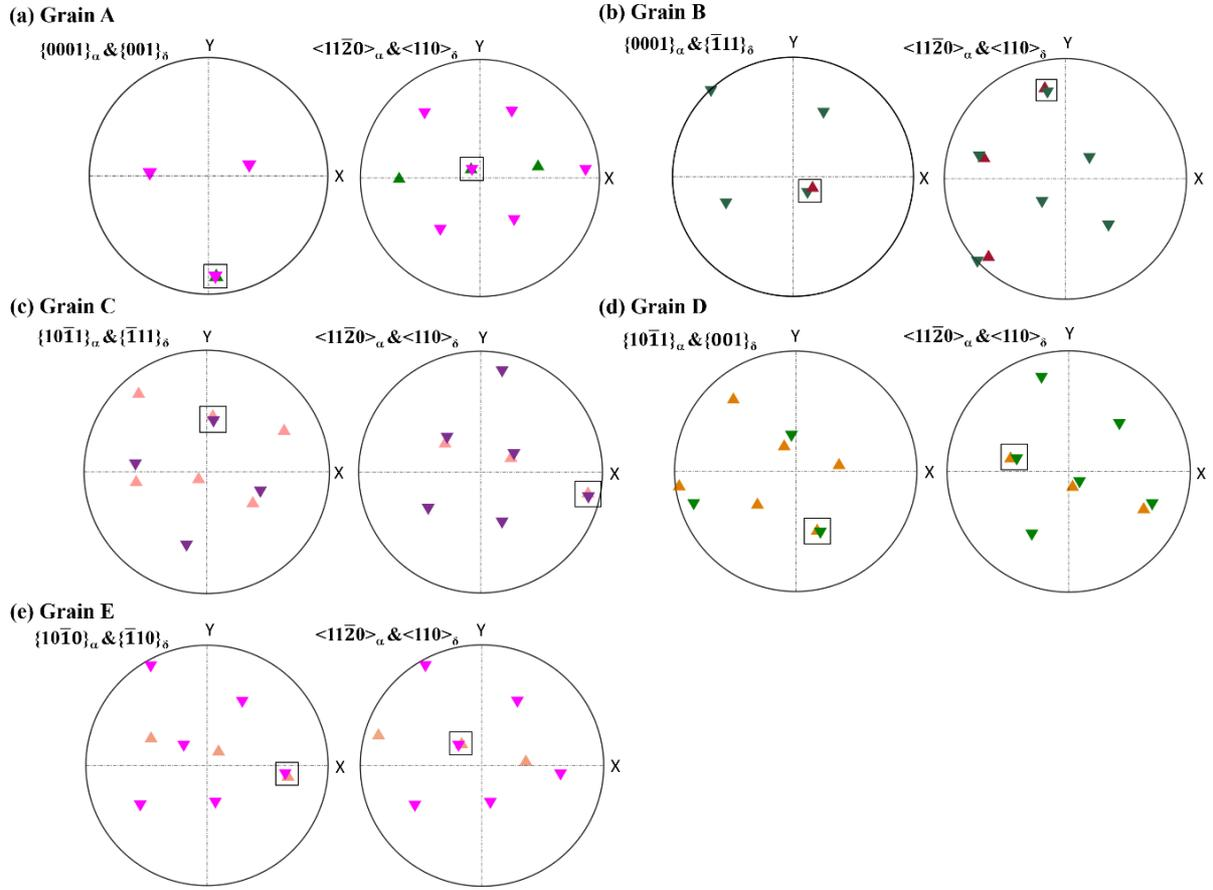
Fig. 4 Stereographic projections of the OR planes and the OR directions corresponding to the matrix  $\alpha$  (hcp) and the hydride  $\delta$ -TiH<sub>2-x</sub> (FCC) in : (a) A grain, (b) B grain, (c) C grain, (d) D grain and (e) E grain (see Fig.3d). The poles of the matrix and the hydride are represented with the consistent colors in (Fig. 3b and d); the coincidences of the  $\alpha$  matrix and  $\delta$ -hydride projections are indicated by the black frames
