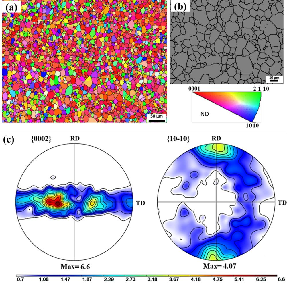
Fig. 1 Initial microstructure of Ti50A revealed by EBSD. (a) Inverse Pole Figure (IPF) map, (b) phase map superimposed with grain boundaries and (c) pole figure of plane  $\{0002\}$  and  $\{10\bar{1}0\}$ , respectively.
