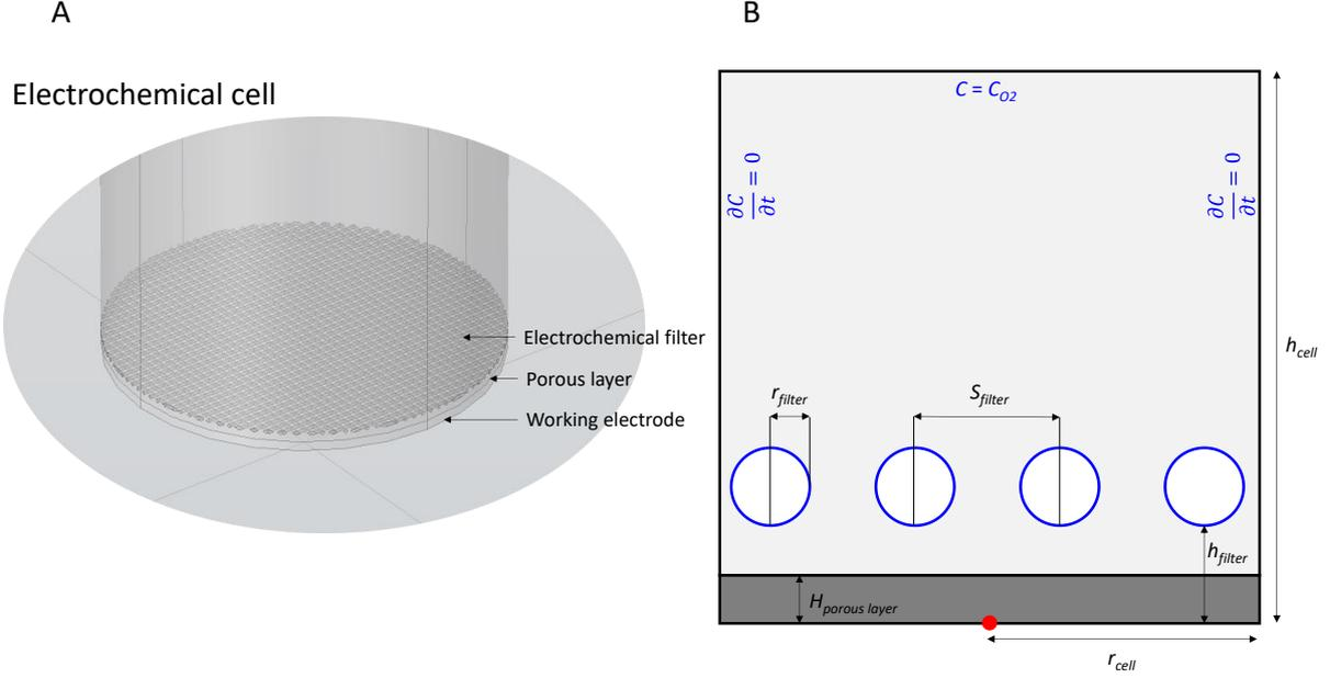
**Figure 1.** (A) 3D representation of the electrochemical cell. (B) 2D representation of the electrochemical cell with the definition of the cell parameters (in black) and of the boundary conditions (in blue). The blue circles represent the Pt wires of the electrochemical wires at which the dissolved oxygen is reduced. The red point is the position at which the dissolved oxygen concentration is calculated (i.e., the surface of the sensor that is associated with this filter).
