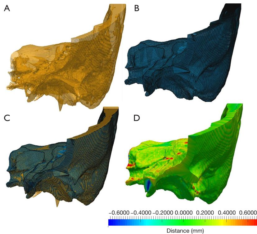
**Figure 5** Example of comparison between rough reconstructed geometry issued from manual segmentation of the DICOM files (A) and the STL mesh files corrected and prepared for 3D printing (B). A superposition of both geometries is given in (C), and a distance map between these two geometries is calculated (D).
