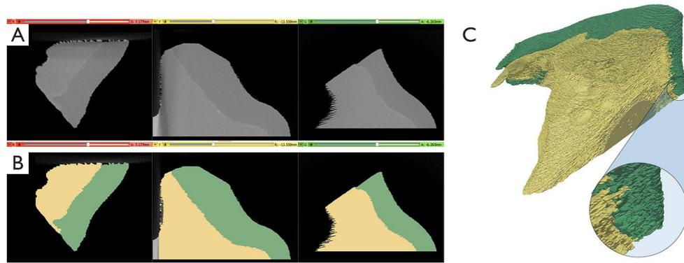
**Figure 4**  $\mu$ CT acquisition (A) and manual segmentation (B) of a fragment of the printed TB model.  $\mu$ CT data are used to generate a 3D model (C) to be compared with the initial STL files sent to the 3D printer.
