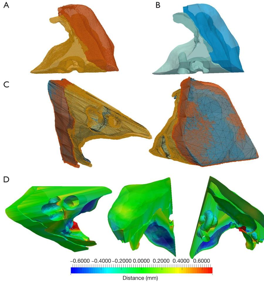
**Figure 8** Qualitative comparison between STL files sent to the 3D printer and the actual geometry of the printed model issued from  $\mu$ CT. (A)  $\mu$ CT reconstruction of soft and hard tissues from the bi-material printed model. (B) Corrected STL files initially sent to the 3D printer, separated into soft and hard tissues. (C,D) Superposition of the geometries before and after printing.
