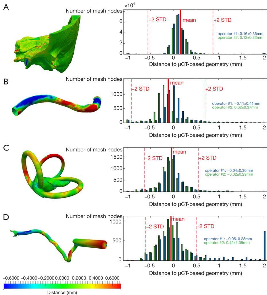
**Figure 6** Distances between the rough reconstructed geometry issued from manual segmentation of the DICOM files and the STL mesh files corrected and prepared for 3D printing, for temporal bone (A), sinus (B), vestibule/semicircular canals (C) and facial nerve (D).
