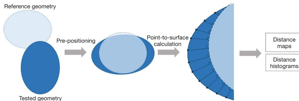
**Figure 3** Explanatory diagram of the point-to-surface distances calculation. “Reference geometry” represents the segmentation of the CT-scan devoid of correction. “Tested geometry” corresponds to the geometry with mesh corrections.
