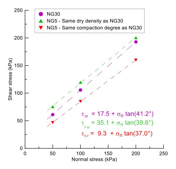
Figure 9: Failure envelopes of NG30 and NG5 (NG30:  $\rho_d = 2 \text{ Mg/m}^3$  and NG5:  $\rho_d = 2 \text{ or } 1.83 \text{ Mg/m}^3$ ).
