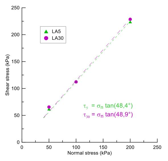
Figure 6: Failure envelopes of LA5 and LA30 at  $\rho_d$  = 1.73 Mg/m<sup>3</sup>.
