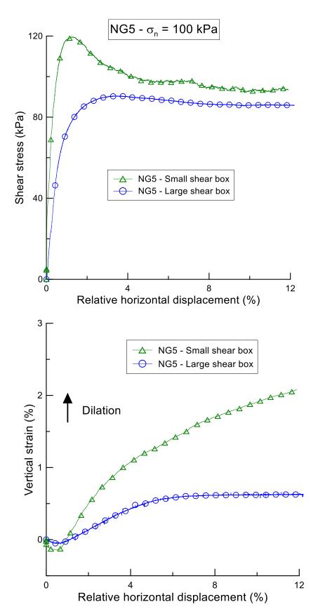
Figure 4: Effect of specimen dimensions on the shear strength of NG5 ( $\sigma_n = 100 \text{ kPa}$ ).
