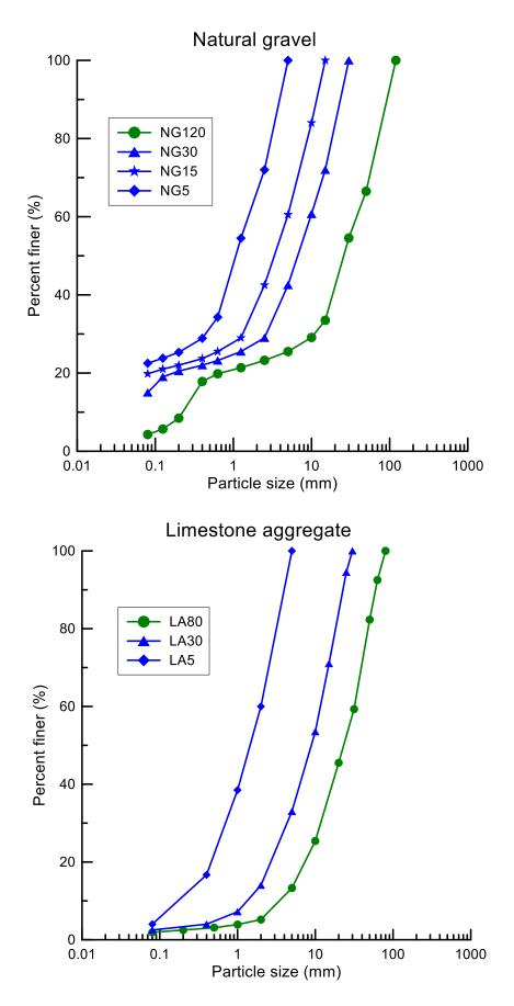
Figure 2: Grain size distribution curves of the studied soils.
