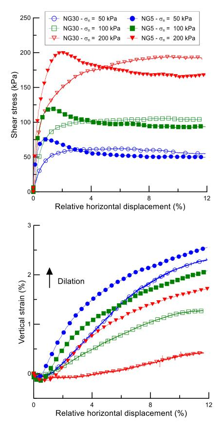
Figure 8: Shear stress-relative horizontal displacement and volume variation curves of NG5 and NG30 at  $\rho_d = 2 Mg/m^3$ .
