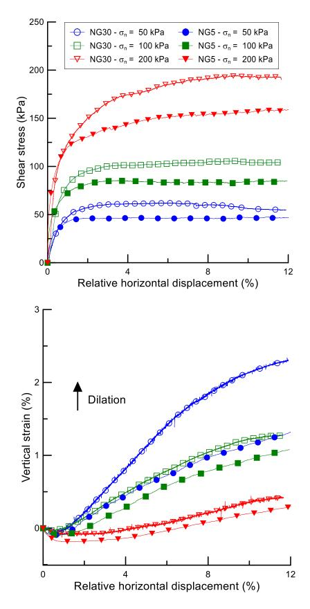
Figure 7: Shear stress-relative horizontal displacement and volume variation curves of NG5 and NG30 at 94% of compaction degree (NG30:  $\rho_d = 2 Mg/m^3$  and NG5:  $\rho_d = 1.83 Mg/m^3$ ).
