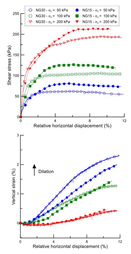
Figure 10: Shear stress-relative horizontal displacement and volume variation curves of NG15 and NG30 at  $\rho_d = 2 Mg/m^3$ .
