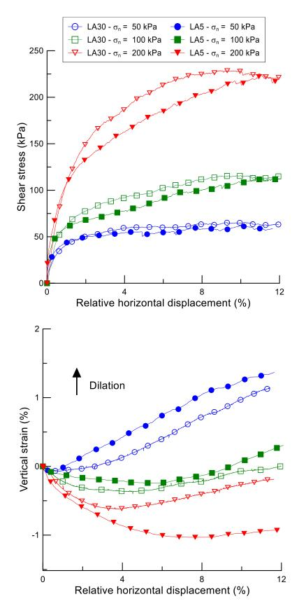
Figure 5: Shear stress-relative horizontal displacement and volume variation curves of LA5 and LA30 at  $\rho_d = 1.73 \text{ Mg/m}^3$ .
