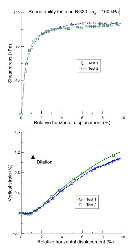
Figure 3: Repeatability tests on NG30 under 100 kPa of normal stress in the large shear box.
