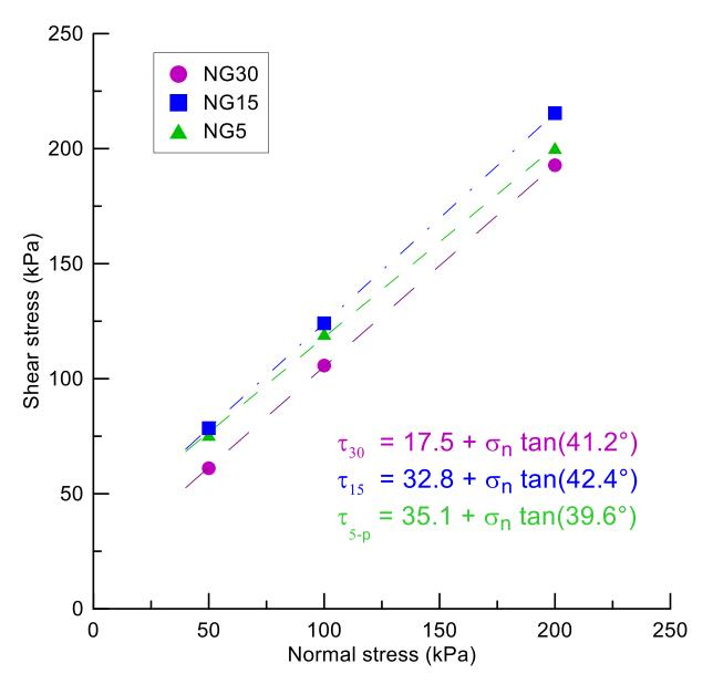
Figure 11: Failure envelopes of NG specimens tested at  $\rho_d = 2 Mg/m^3$ .
