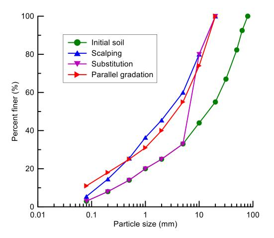
Figure 1: Modification of the grain size distribution curve for the three different approaches (initial soil:  $d_{max} = 80 \text{ mm}$  and reconstituted soils:  $d_{max} = 20 \text{ mm}$ )
