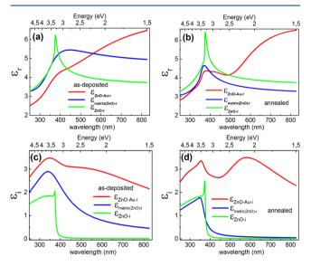
**Figure 6.** Real (a,b) and imaginary (c,d) dielectric functions of a ZnO-Au nanocomposite film of 20% Au, its ZnO matrix, and pure ZnO films for the as-deposited state (a, c) and after annealing in air at 300 °C (b, d).
