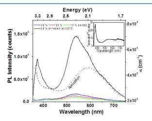
**Figure 8.** Photoluminescence of as-deposited films and film containing 29% Au annealed at 300 °C. The inset shows the ratio of PL intensity of the film containing 29% Au after annealing to the PL intensity before annealing for the same sample.
