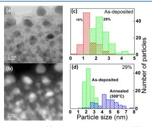
**Figure 2.** Bright field (a) and high angle annular dark field (b) STEM micrographs of a ZnO-Au nanocomposite film with 10% gold. Distributions of nanoparticle size (c) for two gold contents in the asdeposited state (up) and for 29% gold in the as-deposited state and after annealing at 300 °C in air (bottom).
