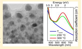
photoluminescence from the ZnO matrix is strongly enhanced upon activation of LSPR showing strong coupling with the gold nanoparticles. Finally, modeling of spectroscopic ellipsometry measurements unambiguously reveals how curing the defects increases the optical bandgap of the ZnO matrix and modifies the optical dielectric functions of the nanocomposite and ZnO matrix.
