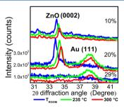
**Figure 1.** X-ray diffractograms of ZnO-Au nanocomposite thin films synthesized with different Au contents (10, 20, and 29%) as-deposited ( $T_{\rm Room}$ ) and after annealing in air at 230 and 300 °C  $\pm$  5 °C.
