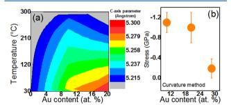
**Figure 3.** 2D contour plot of the c-axis parameter determined using the (0002) ZnO diffraction peak of ZnO and ZnO-Au nanocomposite films as a function of the temperature and the gold content (a). Stress measurements using the curvature method for ZnO-Au nanocomposite films as a function of the Au content (b).
