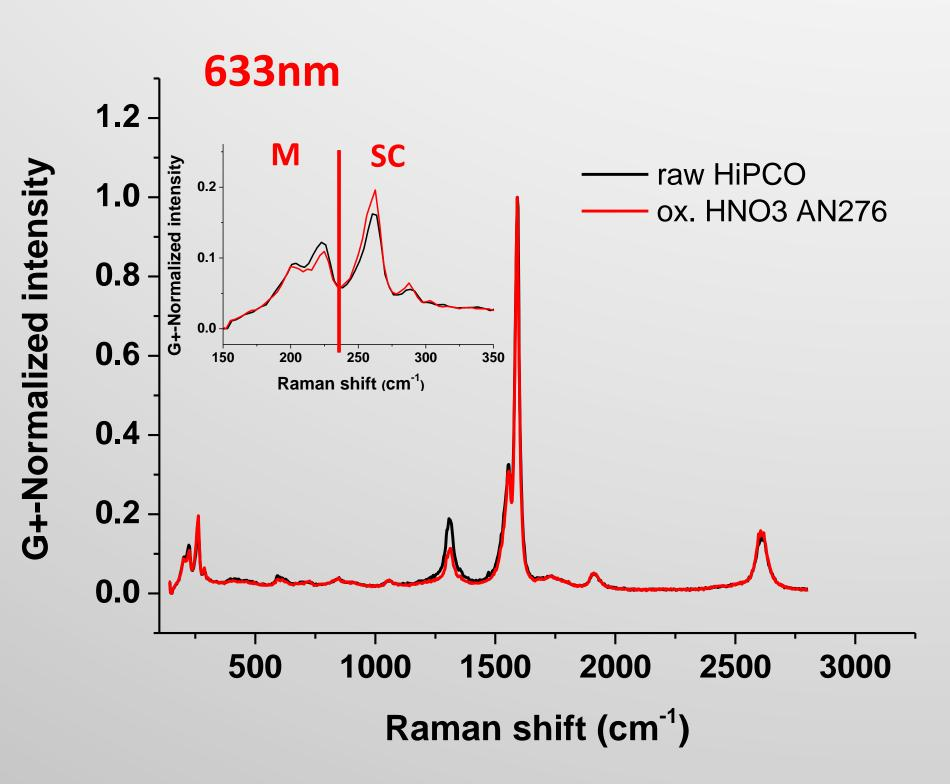
Few defects introduced by HNO<sub>3</sub> oxidation, many defects introduced by radical functionalization with MeOB groups.
