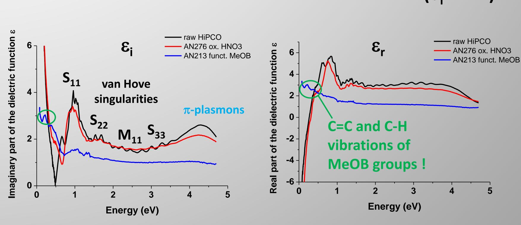
Functionalization strongly decreases the intensity of van Hove singularities and  $\pi$ -plasmon band (but not our microwave-assisted oxidation process). **Detection of MeOB functions!**
