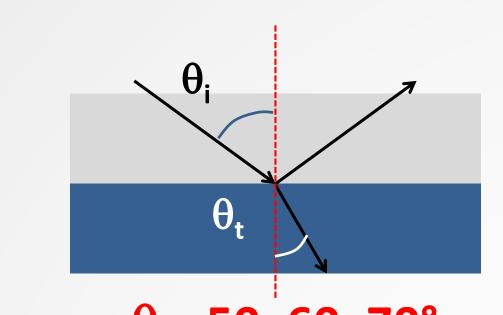
$\theta_i$ : 50, 60, 70° Energy of light: from 0.6 to 4.96 eV and also from 0.07 to 0.6 eV for  $\theta_i = 60^\circ$
