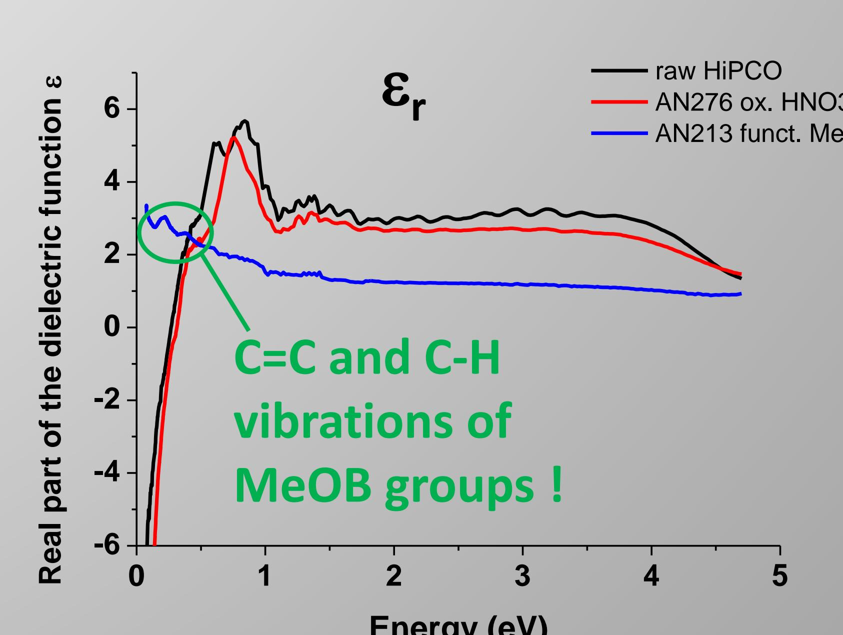
Functionalization strongly decreases the intensity of van Hove singularities and  $\pi$ -plasmon band (but not our microwave-assisted oxidation process).
