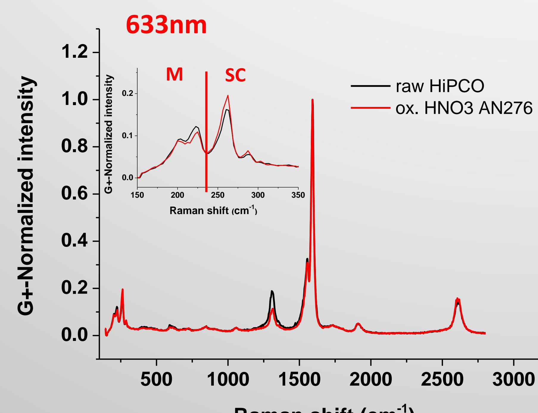
Few defects introduced by HNO<sub>3</sub> oxidation, many defects introduced by radical functionalization with MeOB groups.
