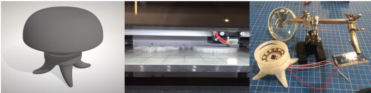
Fig. 4. Decorative interactive object prototypes: 3D model (virtual 3D BDO), rapid prototyping, electronics testing (two stages Stakeholders interactions)
