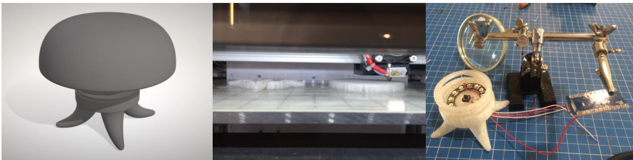
Fig. 4. Decorative interactive object prototypes: 3D model (virtual 3D BDO), rapid prototyping, electronics testing (two stages Stakeholders interactions)
