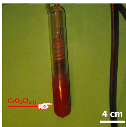
Figure 18. Visual image of the \text{CrO}_2\text{Cl}_2(l) generated during the thermal treatment of chromite by \text{Cl}_2 +air and collected in liquid state at -35^{\circ}\text{C} .
