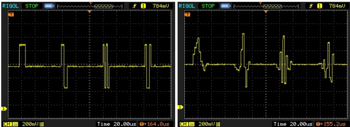
Figure 15: The visualization of transmitted packets by the IDWPT architectures on a FPGA Arty board (Haar wavelet at the left and Db2 wavelet at the right) and 2 levels of resolution.
