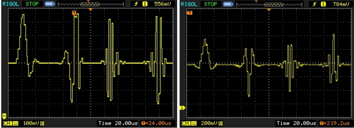
Figure 16: The visualization of transmitted packets by the IDWPT architectures on a FPGA Arty board (Db4 wavelet at the left and Coif2 wavelet at the right) and 2 levels of resolution.
