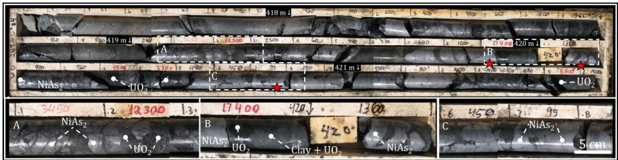
804 Fig. 1 The 417.4 – 421.6 m section of the WC287 drill core, Cigar Lake U deposit (Saskatchewan, Canada). A) 805 Massive U oxide and rammelsbergite vein at 419.1 – 419.3 m depth. B) Association of massive U oxides and 806 rammelsbergite veins at 419.9-420.1 m. C) Rammelsbergite vein at 420.6-420.8 m depth. Red stars correspond to 807 the locations of the three samples analysed (420.0, 420.1 and 420.7). The bottom part of the figure shows an 808 expanded view of each of the three sampled intervals. The number given above each interval of 10 cm is the total 809 counts per second of radioactivity measured by a hand scintillometer. The last sample of a massive rammelsbergite 810 vein was taken from the WC530 drillhole in the Cigar Lake deposit area, at 457.2 m.
