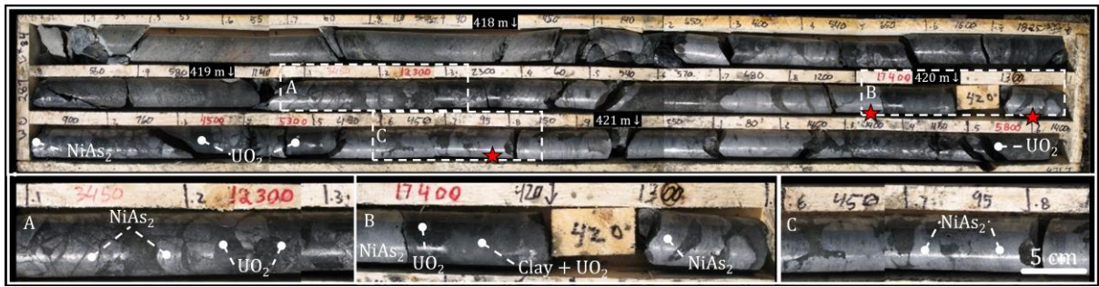
804 Fig. 1 The 417.4 – 421.6 m section of the WC287 drill core, Cigar Lake U deposit (Saskatchewan, Canada). A) 805 Massive U oxide and rammelsbergite vein at 419.1 – 419.3 m depth. B) Association of massive U oxides and 806 rammelsbergite veins at 419.9-420.1 m. C) Rammelsbergite vein at 420.6-420.8 m depth. Red stars correspond to 807 the locations of the three samples analysed (420.0, 420.1 and 420.7). The bottom part of the figure shows an 808 expanded view of each of the three sampled intervals. The number given above each interval of 10 cm is the total 809 counts per second of radioactivity measured by a hand scintillometer. The last sample of a massive rammelsbergite 810 vein was taken from the WC530 drillhole in the Cigar Lake deposit area, at 457.2 m.
