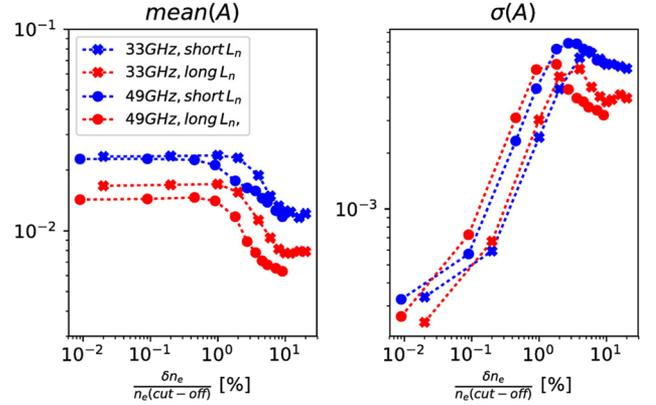
FIG. 12. Average and standard deviation of the reflectometry amplitude  $A(t)$  signals for turbulence level scans in the case of outward radial plasma flow for 2 probing frequencies  $f_p$  and 2 density gradient scale lengths  $L_n$ .
