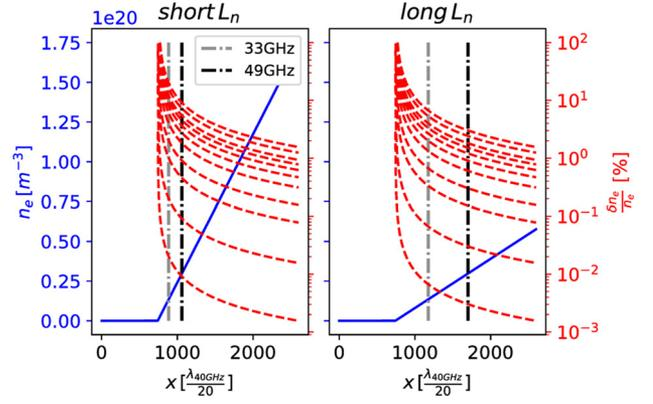
FIG. 2. Linear background density profiles (solid blue) and radial positions of the  $f_p = 33$  GHz and  $f_p = 49$  GHz cutoffs, together with the set of density turbulence level profiles (dashed red) employed for the numerical plasmas.
