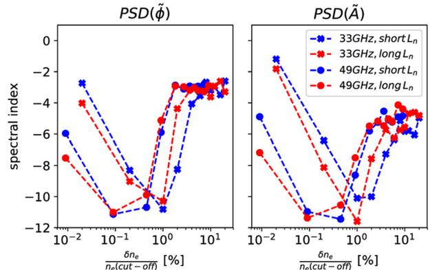
FIG. 5. Spectral index obtained from the fluctuating components of  $A(t)$  and  $\varphi(t)$  signals in turbulence level scans with 2 probing frequencies  $f_p$  and 2 density gradient scale lengths  $L_n$ .
