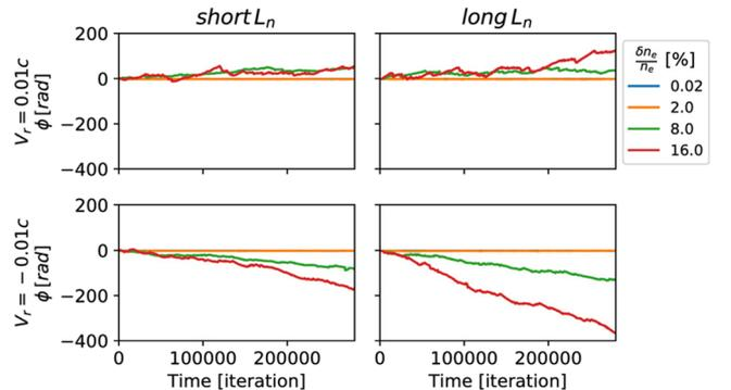
FIG. 10. Time traces of reflectometry  $\varphi(t)$  signals for turbulence level scans with  $f_p = 33$  GHz probing frequency and 2 density gradient scales  $L_n$  for both cases of inward and outward radial plasma flow.
