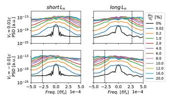
FIG. 9. Power spectra of reflectometry complex amplitude signals  $A(t)e^{i\varphi(t)}$  for turbulence level scans in both inward and outward radial plasma flow directions, with  $f_p = 33$  GHz probing frequency, and two different density gradient lengths  $L_n$  of background *slab* plasmas.
