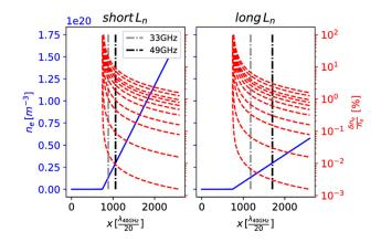
FIG. 2. Linear background density profiles (solid blue) and radial positions of the  $f_p = 33$  GHz and  $f_p = 49$  GHz cutoffs, together with the set of density turbulence level profiles (dashed red) employed for the numerical plasmas.
