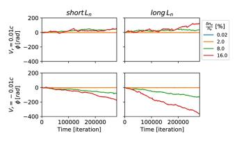
FIG. 10. Time traces of reflectometry  $\varphi(t)$  signals for turbulence level scans with  $f_p = 33$  GHz probing frequency and 2 density gradient scales  $L_n$  for both cases of inward and outward radial plasma flow.
