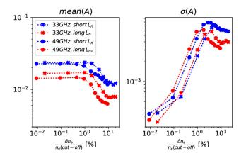
FIG. 12. Average and standard deviation of the reflectometry amplitude A(t) signals for turbulence level scans in the case of outward radial plasma flow for 2 probing frequencies  $f_p$  and 2 density gradient scale lengths  $L_n$ .
