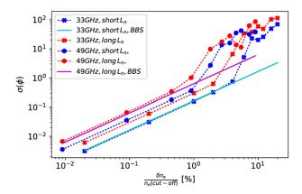
FIG. 11. Standard deviation of reflectometry  $\varphi(t)$  signals for turbulence level scans with 2 probing frequencies  $f_p$  and 2 density gradient scale lengths  $L_n$ , for outward radial plasma flows. Theoretical values estimated from Eq. (1) for two of the simulated cases are also shown in solid lines.
