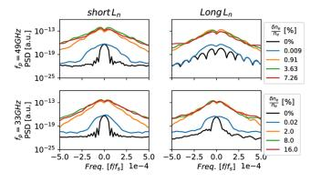
FIG. 3. Power spectra of complex amplitude signals  $A(t)e^{i\varphi(t)}$  for turbulence level scans, in two different density gradient lengths  $L_n$  and two probing frequencies  $f_p$ . Turbulence was generated using a Kolmogorov-like model and set to flow in the poloidal direction.
