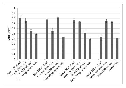
**Figure 5.** Internal bond strength (IB) of tannins-based particleboards. 70 and 100 refer to the extraction tempature of the tannins.
