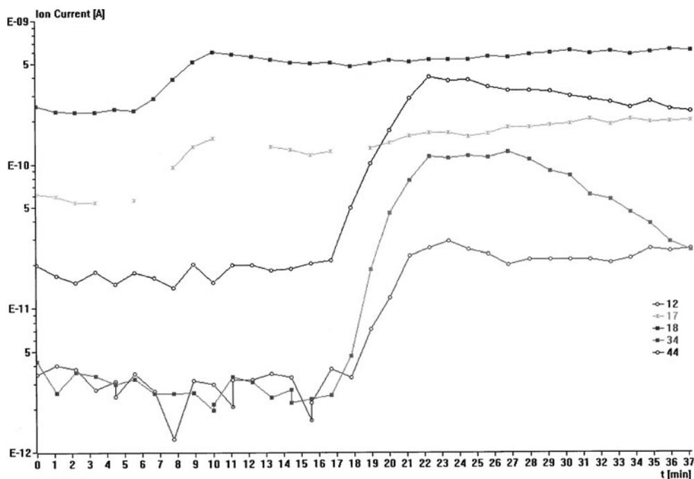
Fig. 4. Mass spectrum of amoxicillin selected molecular ions
