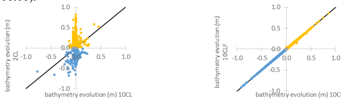
Fig. 7. Cross comparison of simulated bathymetry evolutions between the reference model configuration (10CL) and the two other configurations (2CL and 10CLF). The colours are corresponding to the 10CL's bathymetry evolution: the yellow is the deposition; the grey is the stable bathymetry and the blue is the erosion.
