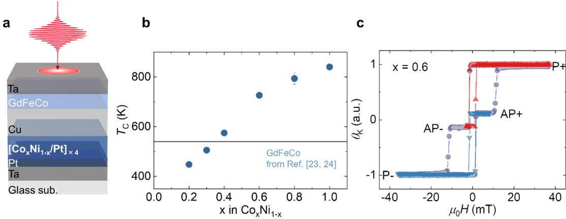
**Figure 1.** Stacking structure and magnetic properties. (a). Stacking structure for the spin-valve structure for AOS measurement. (b). Curie temperature measured for  $[\text{Co}_x\text{Ni}_{1-x}/\text{Pt}]$  multilayers plotted as a function  $x$  (blue symbol). The line corresponds to  $T_C$  for GdFeCo (Ref. [23, 24]). (c). MOKE hysteresis loop measured from film side for  $[\text{Co}_{0.6}\text{Ni}_{0.4}/\text{Pt}]/\text{Cu}/\text{GdFeCo}$  spin-valve structure.
