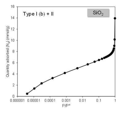
Fig. 4 SiO<sub>2</sub> displaces a mixed nitrogen adsorption isotherm on a semi-log scale.
