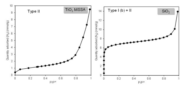
Fig. 3 Characteristic type II nitrogen adsorption isotherm obtained for TiO<sub>2</sub> MSSA and mixed isotherm obtained for SiO<sub>2</sub>.
