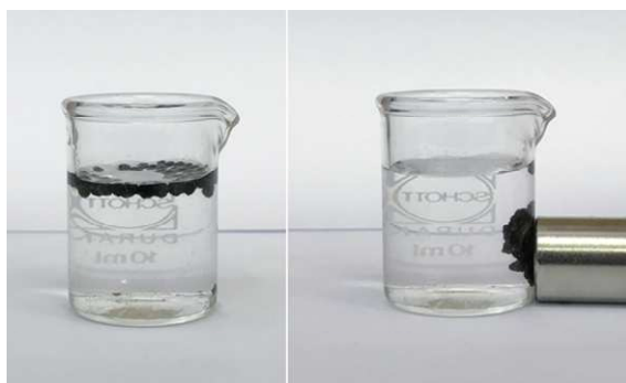
Figure S7. (a) Two sizes of hollow carbon spheres tested as floating bodies for solar evaporation (again chosen broken to reveal their empty character); (b) Evaporation rate of water under simulated solar light without (white bars) and with floating hollow carbon spheres (those based on tannin are coloured in green, no graphitisation catalyst having been used); (c) Strong magnetic character of these spheres when prepared in the presence of iron. (Adapted from [102] with permission from Elsevier).
