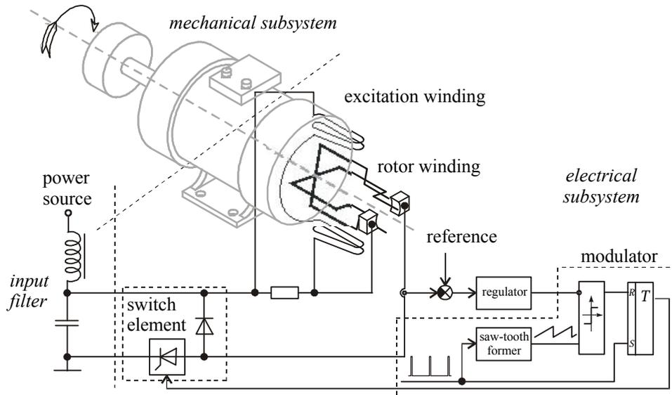
Fig. 1. Functional scheme of the considered electromechanical system
