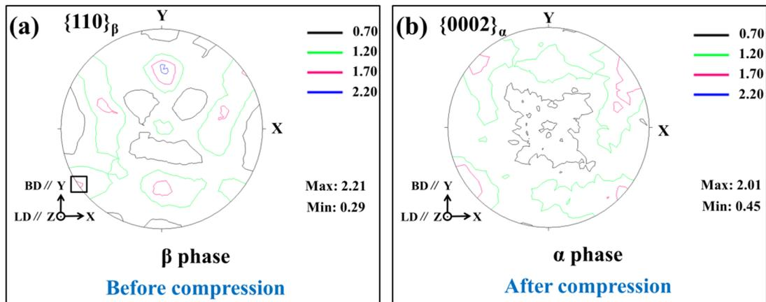
**Fig. A2** (a)  $\{110\}_\beta$  pole figure measured by neutron diffraction at room temperature before the hot compression; (b)  $\{0002\}_\alpha$  pole figure measured after the hot compression. The black frame in (a) indicates the  $\{110\}_\beta$  peak used to detect the formation of the intragranular  $\alpha$  precipitates during *in-situ* neutron diffraction measurement.
