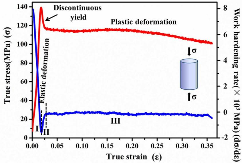
**Fig. 2** Stress-strain ( $\sigma$ - $\epsilon$ ) curve (in red) of the Ti-7333 alloy compressed at 973K to the strain of 0.35 and the corresponding work hardening rate-strain ( $d\sigma/d\epsilon$ - $\epsilon$ ) curve (in blue).
