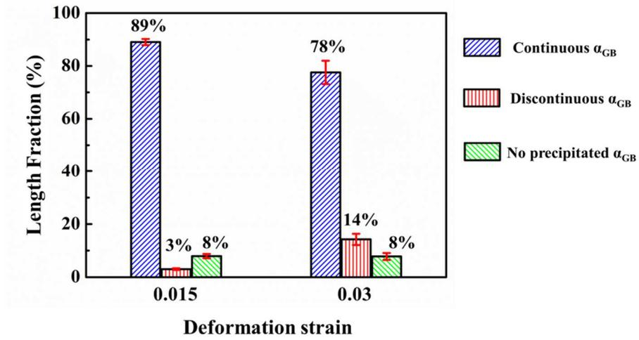
**Fig. 6** Length percentages of  $\beta$  grain boundaries with continuous  $\alpha_{GB}$ , with discontinuous  $\alpha_{GB}$  and without  $\alpha_{GB}$  in the specimens deformed to the respective strains of 0.015 and 0.03. The data are collected from an area of  $2 \times 1 \text{ mm}^2$ .
