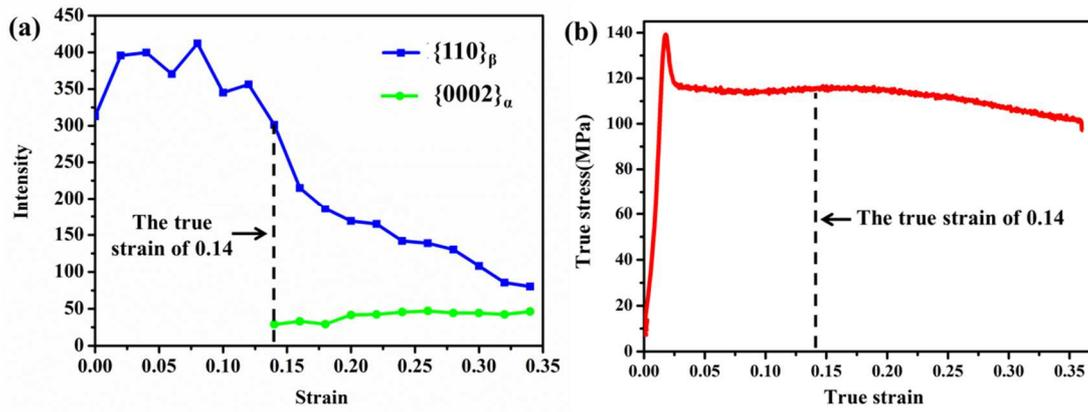
**Fig. 7** Evolution of the diffraction intensities of the  $\{110\}_\beta$  reflection of the  $\beta$  phase and the  $\{0002\}_\alpha$  reflection of the  $\alpha$  phase during the isothermal compression .
