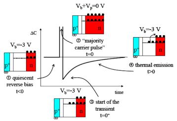
FIGURE 1. Differents phases of DLTS measurement [14]
