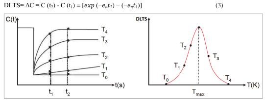
**FIGURE 3.** Evolution of the capacity transient and the DLTS signal ( $\Delta C$ ) vs the temperature, in this example  $T_4 > T_3 > ... > T_0$  [11]
