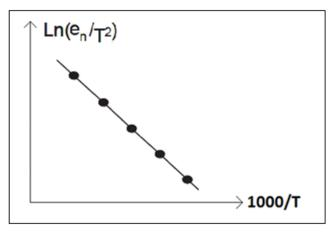
FIGURE 6. The Arrhenius line by the five-points method
