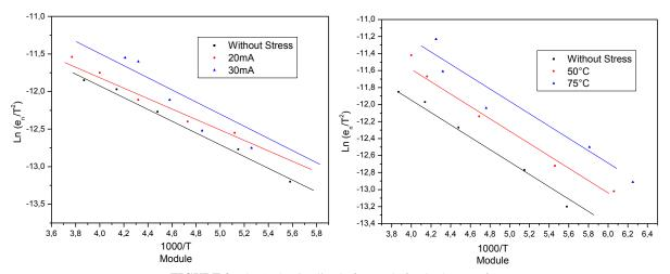
**FIGURE 9.** The Arrhenius line before and after both type of stress
