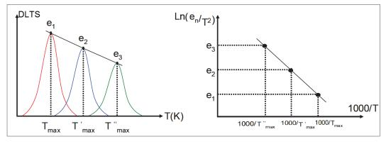
**FIGURE 4.** The Arrhenius line by the Lang's method [3]
