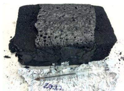
Fig. 1. Mould (left) used for the preparation of tannin-based foams (right).
