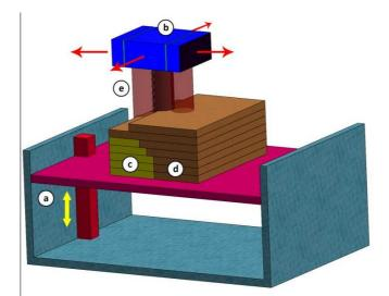
Figure 13: Diagram of the PolyJet process, including (a) vertically movable building platform, (b) multi-nozzle inkjet head, (c) layers of support material, (d) layers of building material, and (e) UV source attached to inkjet head.
