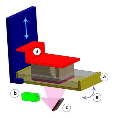
Figure 12: Diagram of the digital light processing (DLP) process, including (a) vat filled with photopolymer resin, (b) light source, (c) micromirror array, (d) vertically movable building platform, and (e) tilting device to replenish the uncured bottom layer. This is a bottom-to-top building process in which a light source solidifies the photopolymer resin in a continuous production method [141].
