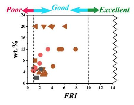
Figure 8: Variation in FRI for PA6 polymer composites containing mineral, carbon-based and metal oxide nanoparticles as a function of weight percent (wt.%). Colored symbols are indicative of the category of the nanoparticles.
