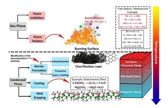
Figure 6: Possible action mechanisms of flame retardants in the gas and condensed phases.
