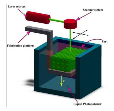
Figure 11: A diagram of Stereolithography (SLA) technology in top-to-down production form. The UV light creates the final object layer by layer in the photocurable resin bath without using any support structure [24].
