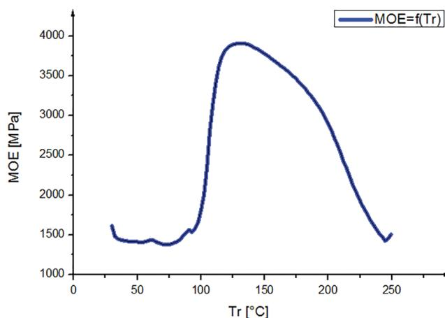
**Figure 4:** TMA curve of the bio resin
