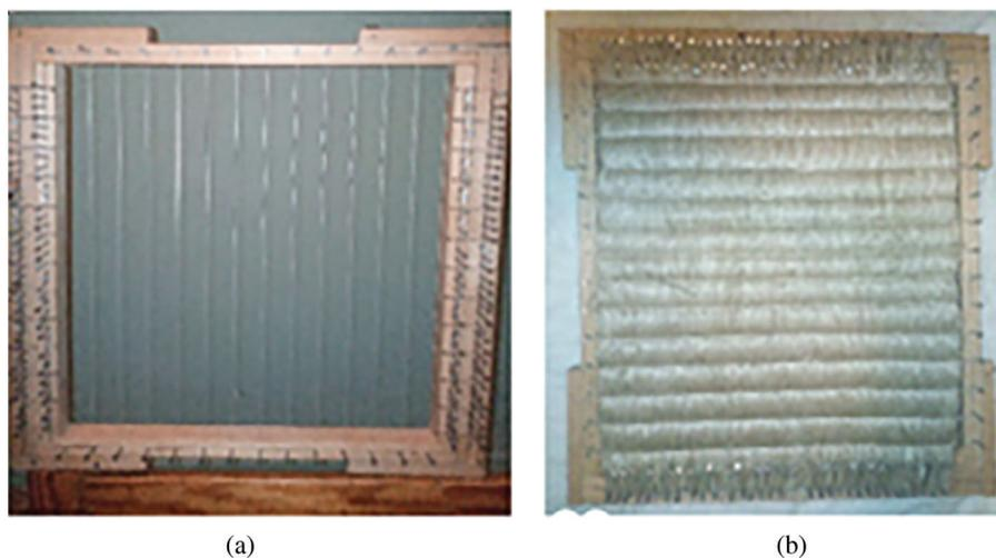
**Figure 6:** (a) Weaving equipment (b) Fiber arrangement
