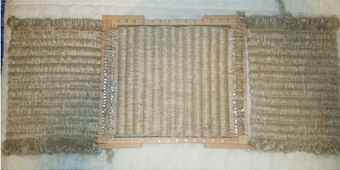
Figure 7: Unidirectional woven mats
