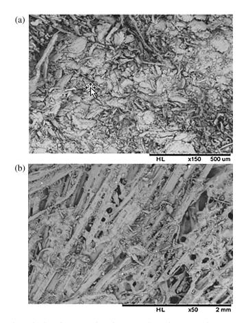
**Figure 9:** Microstructural analysis of composites by scanning electron microscopy (a) cross section view, Gross magnification: 150 and (b) Longitudinal view, Gross magnification: 50
