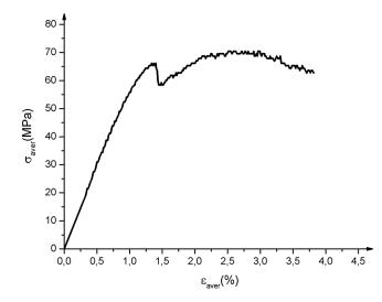
Figure 10: Biocomposites 3-point-bending test average curves.  $\sigma_{aver}$  and  $\varepsilon_{aver}$  are respectively average stress and average strain
