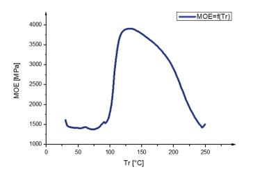
Figure 4: TMA curve of the bio resin
