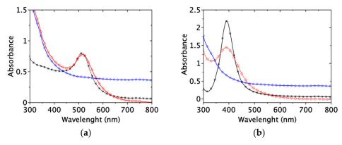
**Figure 5.** UV-visible spectra of 256  $\mu$ mol/L of (a) AuNPs and (b) AgNPs in (\*) water, in (0) CA-MHB, and in (0) CA-MHB after 24 h at 35 °C.
