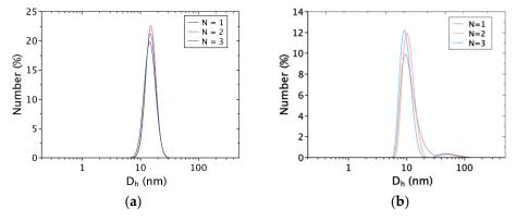
**Figure 2.** Dynamic Light Scattering (DLS) measurements for three independent experiments of (a) the AuNPs and (b) the AgNPs-aqueous solution (102.4  $\mu$ M of metal). Number versus hydrodynamic diameter ( $D_h$ ) in nanometers.
