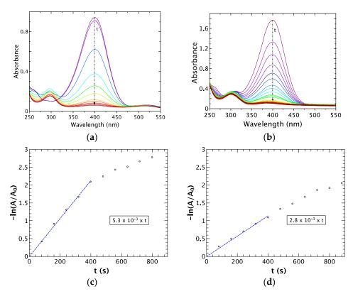
**Figure 4.** UV-vis spectra of 4-nitrophenol reduction as function of time and chemical reaction kinetics determination, respectively for (**a**,**c**) AuNPs and (**b**,**d**) AgNPs (pH = 10; T = 35 °C; 5  $\mu$ g of metal; 10  $\mu$ L of 4-nitrophenol at 1 × 10<sup>-2</sup>  $\mu$ mol/L and 50  $\mu$ L of NaBH<sub>4</sub> at 0.4  $\mu$ mol/L).
